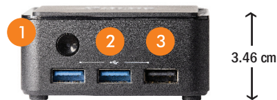
1. Power button, 2. USB 3.2 Port, 3. USB 2.0 Port
