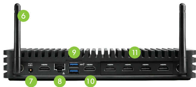
6. Dipole Antennae, 7. Power jack, 8. LAN Port, 9. USB 2.0, 10. USB Port 2.0 11. HDMI Port
