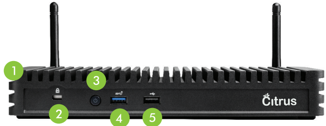
1. Metal Casing, 2. Kensington lock, 3. Power Button, 4. USB Port 3.1, 5. USB Port 2.0
