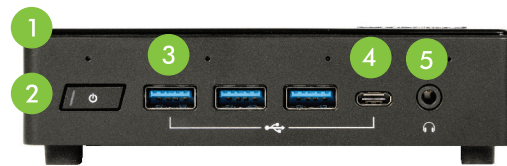
1. Plastic Casing, 2. Power button, 3. USB Port 3.2, 4. C- USB 3.2 Port, 5. Headphone jack
