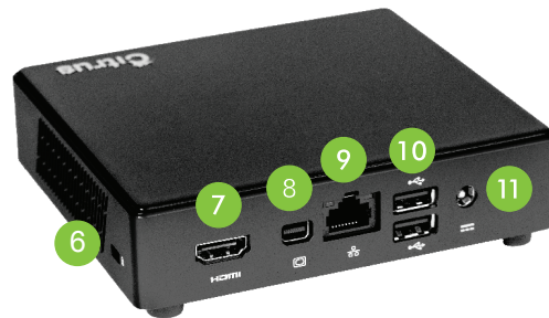
6.Kenington slot, 7. HDMI, 8.Mini DP Port, 9. LAN Port, 10. 2.0 USB x 2, 11. Power Jack
