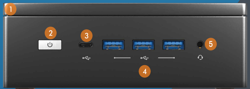
1. Metal Casing 2. Power button 3. USB-C port 4. 3 x USB 3.1 ports 5. Combo Jack
