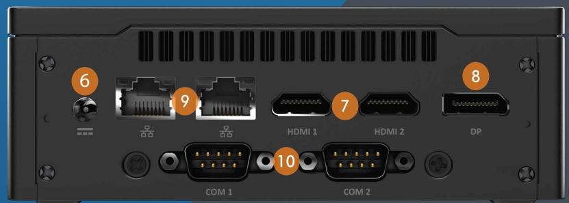
6. Power in 7. 2 x HDMI 2.0 ports 8. Display port 9. 2 x LAN ports 10. 4 x COM ports
